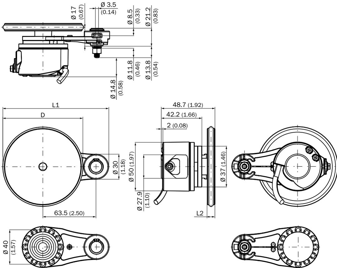
Single wheel, 63.5 mm spring arm, wheel on mounting side, cable connection
