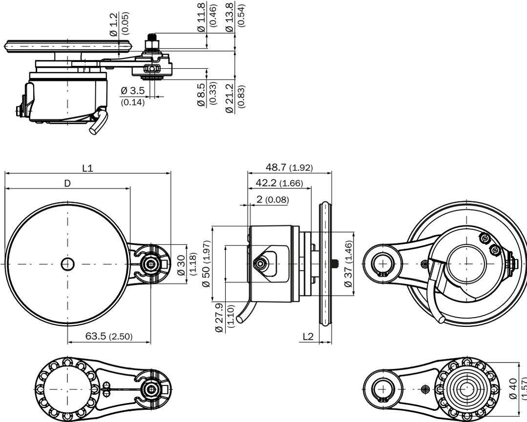
Dual wheel, 12 in, plastic, over-belt yoke mount, connector
