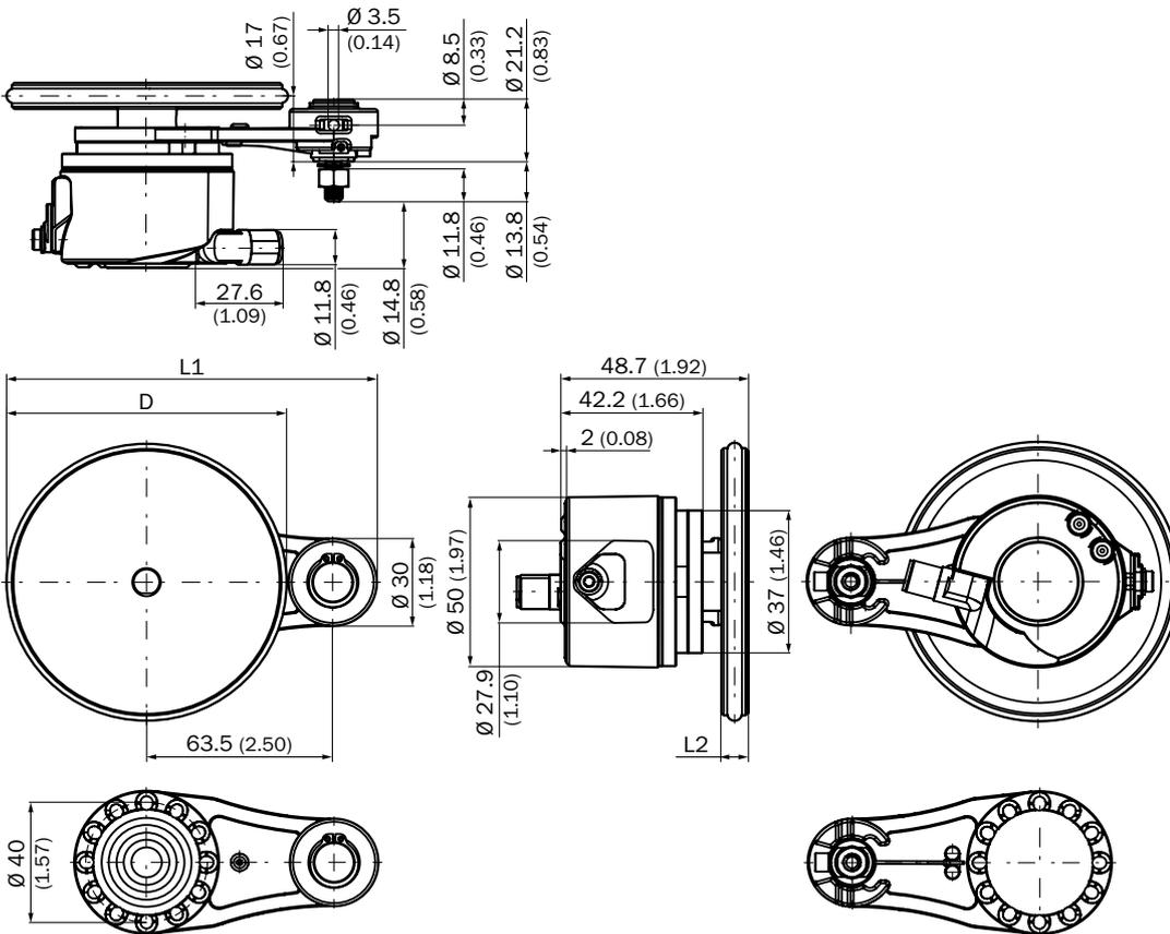
Single wheel, 63.5 mm spring arm, encoder on mounting side, cable connection
