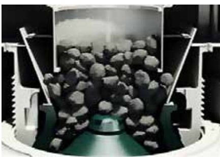
Good feed material level
