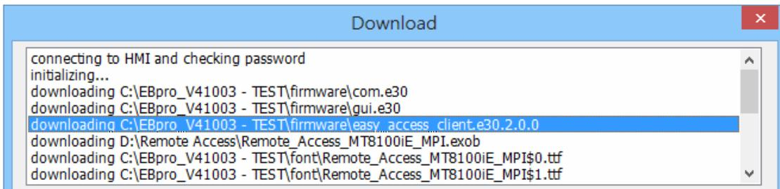
2. The time setting of HMI may be incorrect. If time setting on HMI vastly different from the current time, its security certification will be considered expired and connection will fail.
