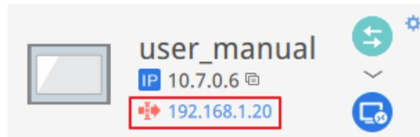
If the remote PLC and the local computer have the same private IP address range, a warning will appear, indicating that subsequent connection to the PLC's IP address will be directed to the remote device instead of the local device if there is any.
