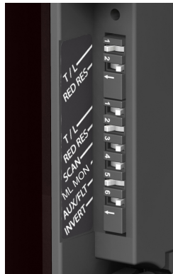
Figure 26. DIP switch settings to program mute configuration options
