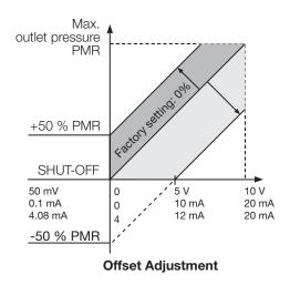
**CAUTION:** Outlet pressures above the maximum outlet pressure (PMR) are not controlled by the valve, i.e. the max. outlet pressure is limited to the PMR.
