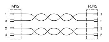
\*The use of a shielded cable is recommended.
