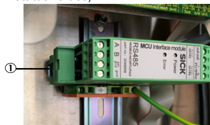
① Hat rail lock ② Ribbon cable connector
