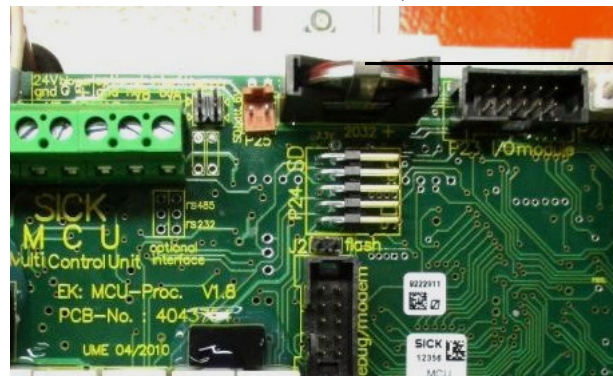
Fig. 64: Replacing the MCU button cell
