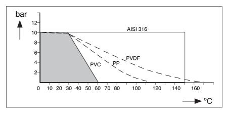
Figure 2-2. Pressure/temperature class
