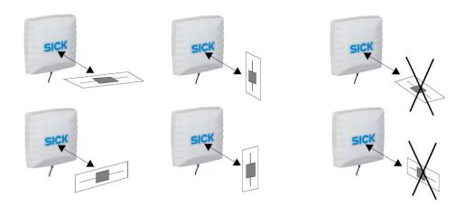
Figure 7: The optimal orientation of the transponder for good writing and reading results is demonstrated here for an external UHF antenna
