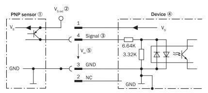
Figure 25: Wiring of digital input "Trigger", supply of trigger sensor by external voltage
