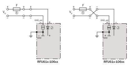
Figure 23: Reversal of the polarity of the supply voltage: no effect on the RFID device (see requirements)
