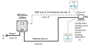
Figure 12: Block diagram RFU61x-106xx (power and Ethernet connection): service operation, e.g. display of read result
