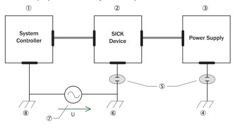
Figure 11: Example: Prevention of equipotential bonding currents in the system configuration by the insulated mounting of the device
