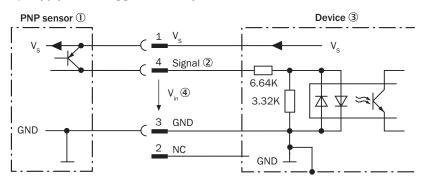
Figure 24: Wiring of digital input "Sensor 1", supply of trigger sensor by the device
