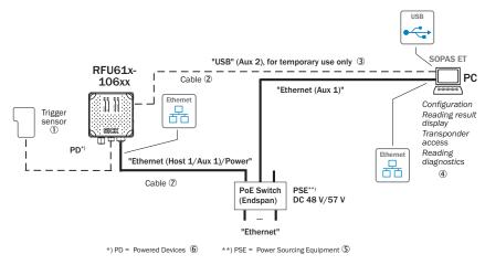
Figure 22: Initial commissioning: connection block diagram RFU61x-106xx (Power over Ethernet)
