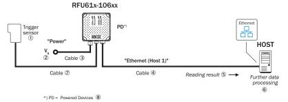
Figure 13: Block diagram RFU61x-106xx (power and Ethernet connection): read operation
