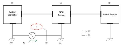
Figure 9: Example: Occurrence of equipotential bonding currents in the system configuration
