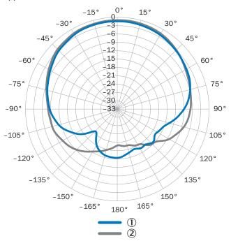
Figure 4: Radiation pattern of the integrated antenna of the RFU61x (typical): Measured antenna gain in dBic at 866.5 MHz, LHCP (left-hand circularly polarized)
