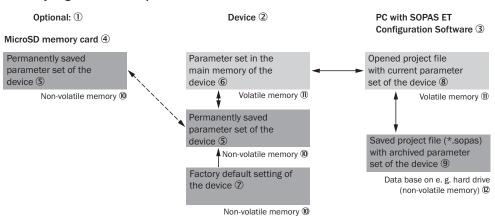
Figure 26: Saving the parameter set and configuration using SOPAS ET
