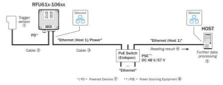
Figure 15: Block diagram RFU61x-106xx (PoE connection): read mode
