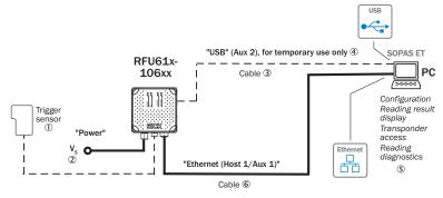
Figure 21: Commissioning: connection block diagram of the RFU61x-106xx (power and Ethernet)
