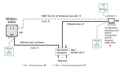
Figure 14: Block diagram RFU61x-106xx (PoE connection): service operation, e.g. display of read result
