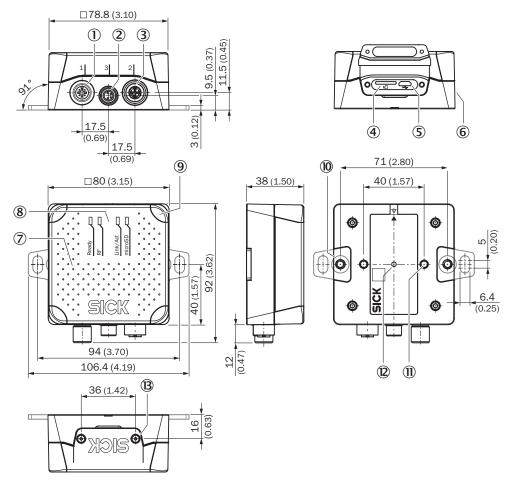
Figure 3: RFU61x-106xx: Structure and dimensions, unit: mm (inch), decimal separator: period
