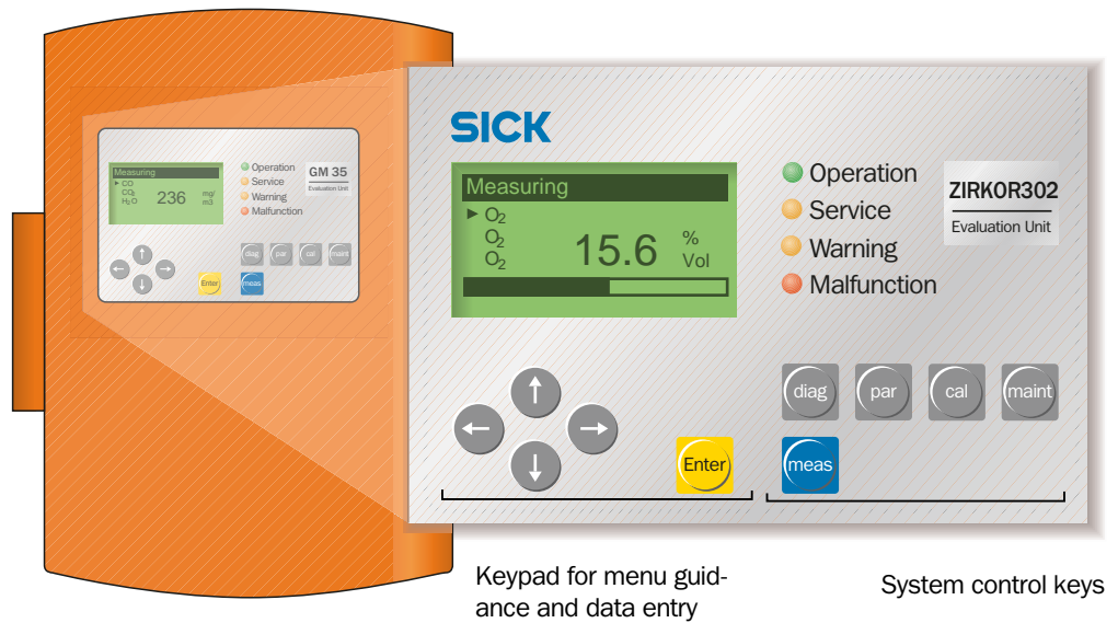
Fig. 10 Indicators and controls on the Evaluation Unit (cast aluminium shown here)
