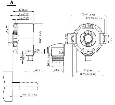
Through hollow shaft, connector outlet - standard system
