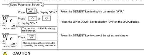
If the burnout action setting is changed, the wiring resistance correction is automatically set to OFF (0). Correct the wiring resistance again after changing the burnout action setting.
