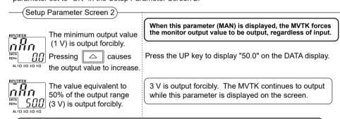
After completion of the forced output, return the MON parameter setting to "OFF" (making the adjustment screen invisible).
