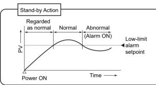
If an alarm type code with stand-by action is set, alarm action is turned off during the start-up control.
