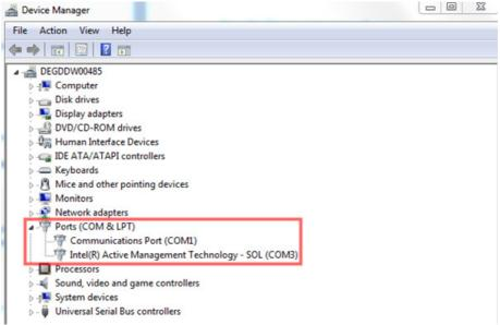
6 Now connect the MCU with the laptop/PC. A new COM port is shown.
