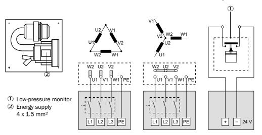
Connect protective conductor to terminal.
