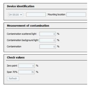
▶ If the measured values for contamination, zero point and span are within the allowed ranges, save them to the device by clicking the "Refresh" button ("Check values" field); if not, repeat cleaning and check the contamination value again by triggering a renewed function check.
