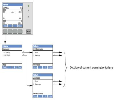
"Diagnosis / Error messages/warnings" provides detailed information on the current device state. To display, connect the measuring system to SOPAS ET and start the device file "DH SB50", "DH SB100" or "MCU".
