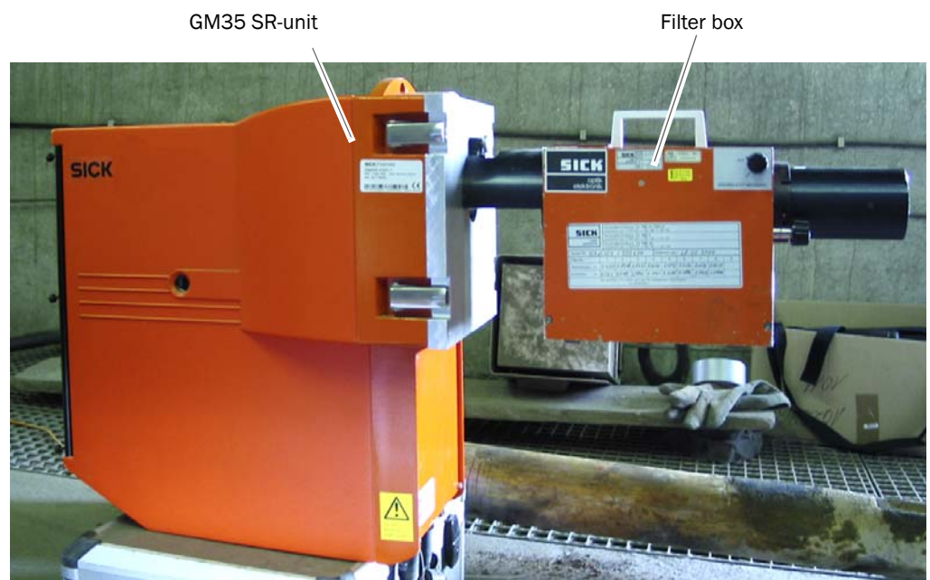
Fig. 67: Installing the filter box
