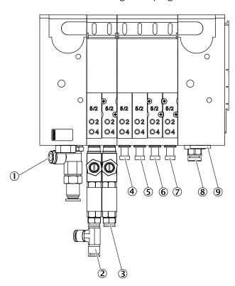
Gas connections of the gas sampling unit hose bundle line
