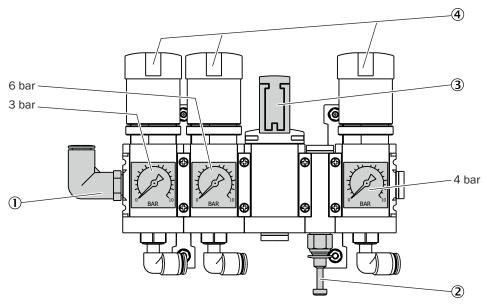
Figure 10: Pressure reducer module
