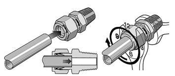
Figure 8: Clamping ring screw connection
