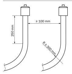
Figure 7: Sample gas line: Distance and radius
