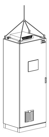
Figure 6: Analyzer cabinet suspension
