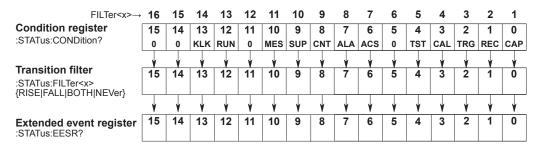
The meaning of each bit of the condition register is as follows:
