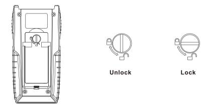
Insert two AA batteries into the holder following the polarity markings. Always close the cover after installing batteries.
