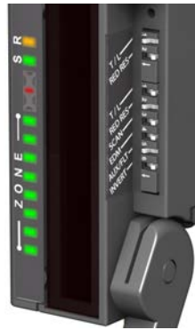
Figure 50. DIP switch configuration to enable cascade installation
