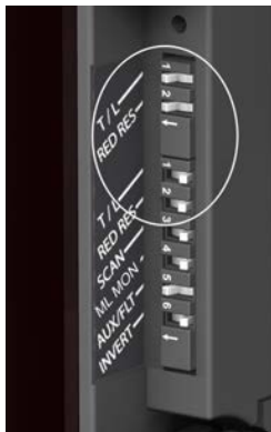
Figure 27. DIP switch configuration to teach fixed blanking
