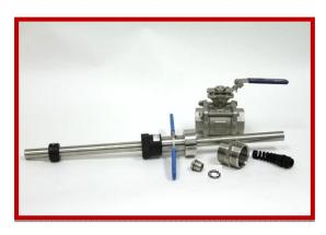
2. Unscrew and remove the sensor tip from the holder, and take O-ring that was in the bag with the Instruction Manual and install it onto the sensor tip as shown.
