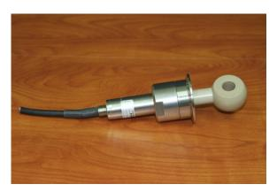
7. Slide the plastic nut onto the ISC40G(S)-GS sensor and thread it onto the back of the sensor body as shown in the image to the right. Installation of the fitting onto the sensor is now complete.
