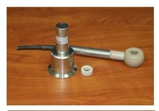
2. Unscrew the sanitary fitting pieces and locate the O-ring (A) and a metal sealing ring (B).
