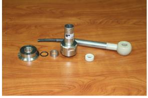
3. Slide the tri-clamp piece onto the ISC40G(S)-GS sensor, followed by the o-ring and then the metal sealing ring.
