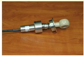
5. First thread the back portion of the tri-clamp fitting into the front tri-clamp piece ensuring a snug fit, as shown in the image to the right.
