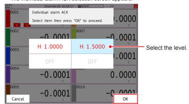
3 Select the level to acknowledge, and tap OK. The alarm output is released.
