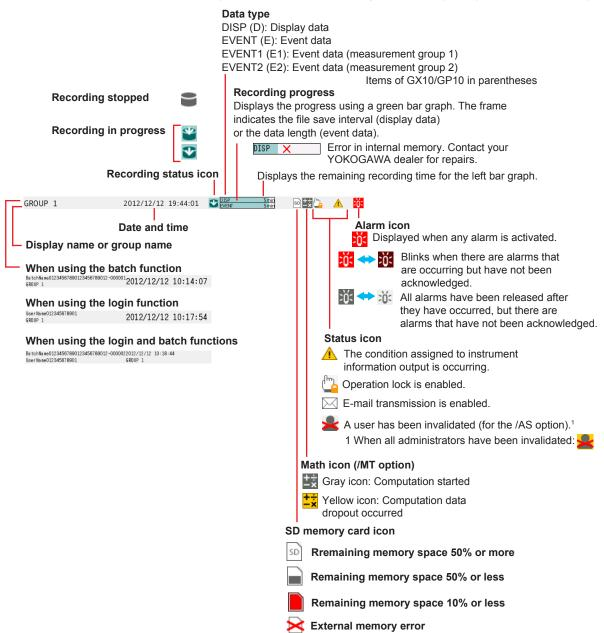
Recording Status Icons When the Program Control Function (/PG option) Is Enabled
