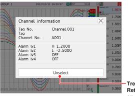
Trend display Returns the waveform displayed on top to the original condition.
