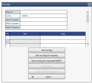
3 Click Start recording or Start recording and computing. Recording starts. The indicator below the Recording button turns on.
