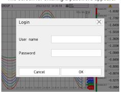
**3.** Enter the user name and password, and then tap **OK**. You can now operate the GX/GP. The user name is displayed in the status display section. The password that you enter is displayed as a string of asterisks.
