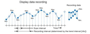
The measured data of display data is divided at the interval specified by the **saving interval** and saved to files.
