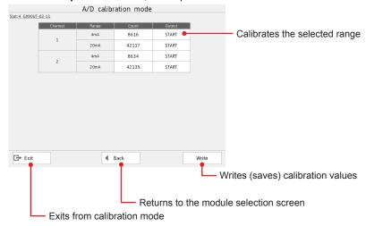
7 Tap **START** for the 4 mA range of the channel to be calibrated.
