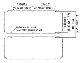
Unit: mm (approx. inch) Unless otherwise specified, tolerance is ±3% (however, tolerance is ±0.3 mm when below 10 mm).
