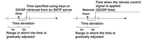
Example: When changing the time to 12 hours 55 minutes 35 seconds when the internal clock is 12 hours 55 minutes 32 seconds
