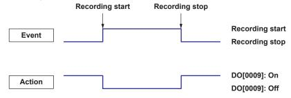
This example assumes that a DI/DO module is installed in slot 0 of the GX/GP main unit. Use event action numbers 4 and 5.
