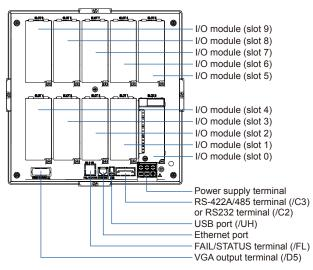
Precautions to Be Taken While Wiring With a screw terminal, we recommend that you use a crimp-on lug with an insulation sleeve (M4 for power supply wiring, M3 for signal wiring).
