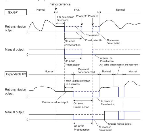
1 When the LAN cable is disconnected, the previous value is output for 5 seconds. When 5 seconds elapse, preset action on error is performed. If the connection recovers, the output is resumed.
