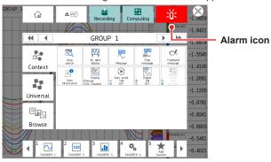
3 Tap OK. The alarm output is released.
