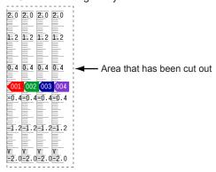
To align the scale position to the positions where the value indicator marks will appear, create guidelines. The lines marked in red on the scale are the guidelines. Erase everything except for the lines marked in red. This image will be used as the base of the scale image.
