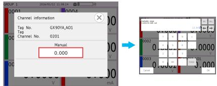
3 Set the output value, and tap OK. The specified value is output.
