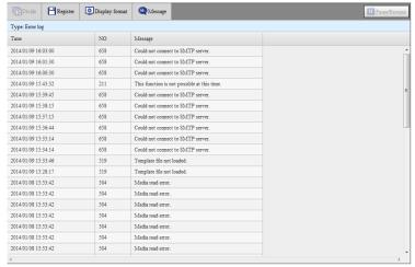
You can sort, rearrange columns, change column widths, and copy to clipboard. The maximum number of log entries is shown below.
