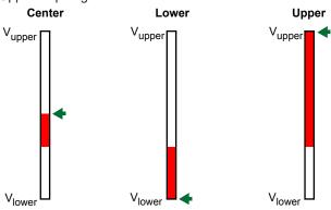
Vupper: Span upper limit (or scale upper limit) Vlower: Span lower limit (or scale lower limit)
