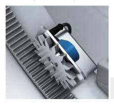
The redundant blade angle monitoring function makes it possible to check whether the rotor blades actually turn when the pitch motor is rotating. The
