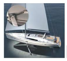
Alignment of the keel is automated on modern sailing yachts. Depending on the water depth e.g. near the coast or in waters with varying sandbanks, the keel can be damaged or the ship may even run aground. Exact position determina-
