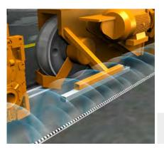
The position of the crane must be detected automatically. Outdoor use and long distances present substantial challenges to the measuring system, often charac-
