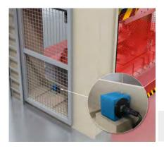
To determine the position of the press stroke, a BKS wire draw encoder is used. It reliably supplies signals for establishing the top dead center (TDC) and bottom dead center (BDC).v
