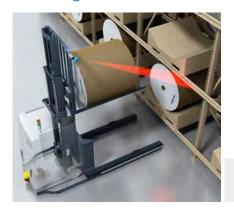
The CLV650 bar code scanner reads the bar code at the shelf and delivers the data to a central computer. This assigns the corresponding path to the automated guided vehicle (AGV) to incorporate the paper roll into the production process as scheduled. The autofocus function
