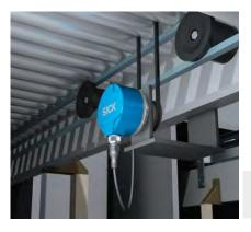
The conveying speed of a roller conveyor is controlled with the help of the position detection feature of a DBS60 programmable incremental encoder. With its high 16-bit resolution, the encoder ensures maximum reproducibility. The encoder
