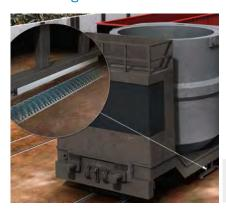
Proper positioning of outdoor rail-mounted transfer cars and product shuttles during the material handling process is simple with the help of a linear encoder. The encoder's several magnetic heads are buried in concrete between the shuttles' rails while the encoder is mounted underneath the moving shuttle. The
