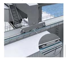
The KH53 is perfectly suited for positioning the traveling trolley on a crane. It provides good repeatability of up to 0.3 mm, and long reading distances of up to 55 mm. It is extremely rugged in the event of shocks and vibrations, and stands up to the affects of severe weather. With the position data of the traveling crane, it is
