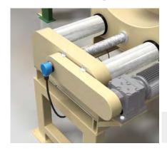
The positioning of saw-blades for setting to the thickness to be sawed is done with the ATM60 absolute encoder. The
