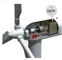
Generally, incremental encoders are used to monitor the rotor speed. These are normally fastened to the hub of the rotor. The DFS60 incremental encoder is used around the world under the harshest conditions. Its stable construction with enclosure rating up to IP67 makes
