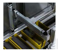
A handling system can be controlled safely and precisely by using the MPA analog positioning sensor. Depending on the drive concept, a compact, high-reso-
