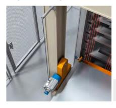
The material lift is used to move stacks of sheets from a transfer carriage or residual sheets from a vacuum nozzle to an interim shelf for storage. The BTF13 wire draw encoder signals the absolute
