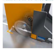
The route of the automated guided vehicle (AGV) is stipulated by the higher-level control system. The DFS60 incremental encoder determines the speed of the
