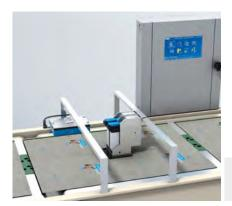
After punching and separating the sheets, the print unit must print a 1D code on each sheet. The SPEETEC 1D non-contact motion sensor fulfills two requirements that are important for this. It detects the speed of the sheet to con-
