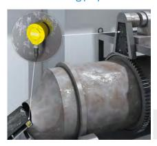
The recycling process for aluminum includes treating any slag, also referred to as dross, produced during the smelting process. This still contains a significant quantity of aluminum that is worthwhile recovering. This slag treatment occurs in rotary kilns that are fed by
