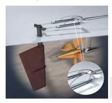
If a new course is to be taken, then the rudder position must be changed to the new direction. The rudder blade is moved by hydraulic cylinders. Linear encoders integrated in the hydraulic cylinders give  $\mu$ m-exact feedback on the position change and therefore the position of the
