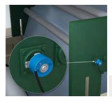
The DBS60 incremental encoder monitors the speed of the film sheet on a roller. This enables the film sheet to be
