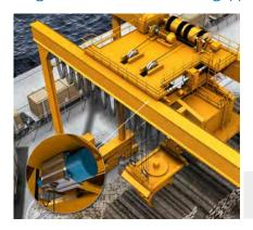
The high-resolution HighLine wire draw encoder measures the height position and speed of the crane gripper. Thanks
