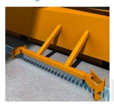
The position of the stacker must be determined automatically. Outdoor use across long distances and under sometimes difficult measurement conditions, such as uneven measuring distances like railways, poses a great challenge to the measuring system. The KH53 linear encoder measures a distance of up to 1,700 m, even under poor environmen-
