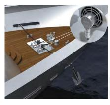
The AFM60 Inox absolute encoder reliably measures the length of the unrolling or cast-out anchor chain. This information is used to brake the anchor winch in good time before reaching the end of the chain. This measurement prevents
