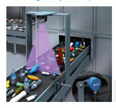
Convyor belts transport waste in recycling planta. A conveyor belt malfunction can cause significant delays in production and involve major costs. It is therefore necessary to monitor the operation of all conveyor belts, as well as the proper loading, unloading, and positioning of
