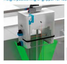
The risk of material breaks in expensive semiconductor wafers must be kept as small as possible. Therefore, the wafer box is monitored with sensors. The Ecoline product family of wire draw en-
