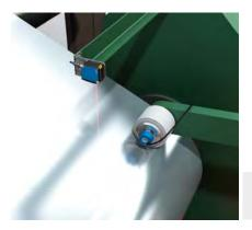
During the finishing process, steel is wound into coils. These are monitored and measured to ensure that the length and width are correct before leaving the winding area. A combination of SICK solutions allows this task to be performed with ease. A LiDAR sensor monitors the width of the coil on the winding
