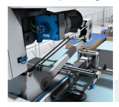
The BCG wire draw encoder supports logistical processes in the large panel warehouse. The encoder detects the exact lift height of the vacuum gripper, which is used for the automated picking
