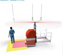
For personal protection and collision prevention with other vehicles or materials on the floor, automated guided systems AGS are equipped on the fork side and on the back wide with safety laser scanners. The AGS is equipped with two drive units with one DBS60
