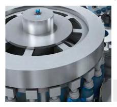
The process of dispensing labels is synchronized with bottle transport, to ensure the label is attached smoothly and in the right place. The labeling module needs to have exact measured values relating
