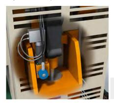
Once the tools have been replaced, the press stroke must be adapted using a primarily mechanical adjustment mechanism. The procedure for adjusting the height of the press stroke can be done
