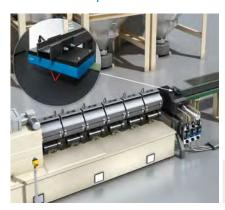
When extruding tire rubber, the belt speed must be controlled so that the rubber does not stretch. This ensures consistently high product quality. For this purpose, the speed at which the tire material reaches the conveyor belt and the continuous advance of the rubber on the conveyor belt must be precisely synchro-
