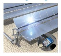
In this system, the sunlight is concentrated by using parabolic mirrors. The sunlight, which enters the mirror parallel to its plane of symmetry, is focused along the focal line and is warming up a heat transfer media like oil. The position of the mirror needs to be guided to follow the sun's daily path in order to achieve
