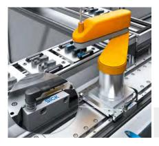
A linear motor moves the SCARA robot synchronously to the conveyor belt so that the robot can pick up workpieces with precision. Without making contact, the TTK70 linear encoder determines the absolute position of the robot. The compact read head of the encoder measures the position on coded magnetic tape reference material without causing
