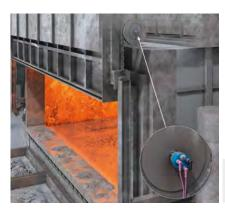
For optimal operation of the collection and holding furnaces, it is also necessary to reduce the cost of heating the furnaces. The position of the furnace door should therefore be monitored to determine whether it is open or closed. If continuous values of the door position are required, the A3M60 PROFIBUS or AFS/
