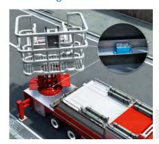
In order to be able to transport people steadily and horizontally, the two-dimensional TMM61 inclination sensor detects the inclination of the basket and forwards this regulation information to
