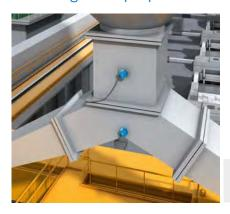
A conveyor pipe distributes the enriched aluminum oxide into various supply bins. The charging cranes in turn take material out of these bins to fill their own bins. The electrolysis cells are supplied by means of the cranes. A mechanical flap determines which storage container the main conveyor pipe will fill. To ensure this
