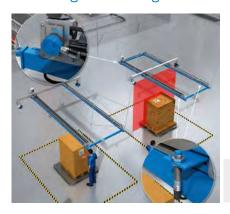
Two LMS5xx 2D LiDAR sensors are installed on a positioning unit above the cargo. This positioning unit is evenly maneuvered along over the cargo, during which two-dimensional scan data of the cargo is recorded. In addition, a DFS60 incremental encoder provides precise speed information. This makes
