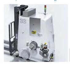
With automated guided systems, the SSM (safe speed monitor) or SLS (safely-limited speed) function monitors the speed on the wheels using the DFS60S Pro encoder and reduces it via the
