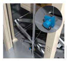
The scissor lift table is positioned using a high-resolution wire draw encoder with a teach-in function. The extremely reliable wire draw encoder does not require
