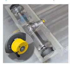
The measured values of the DFS60 programmable incremental encoder control the positioning and speed. With its high resolution, the DFS60 encoder ensures maximum repeatability. There are numer-
