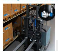
The EcoLine wire draw encoder, which can be compactly integrated into the lifting gear, allows accurate, quick, and reliable measurement of the fork height.
