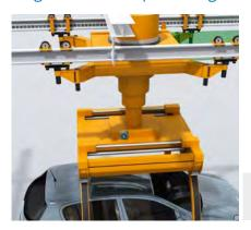
The electrical overhead conveyor brings the car bodies to designated workplaces. The compact BCG wire draw encoder ensures that the defined height position is approached accurately. Eliminating the coupling between the wire draw encoder and suspension mechanism enables highly accurate positioning.
