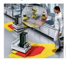
The direction of travel and speed of the transport cars must be recorded to ensure that automated guided carts manage curves quickly and safely. The DFS60S Pro safety encoder and the Flexi Soft safety controller with the FX3MOC motion control module from SICK are ideal for this application. This safe system solution can also be integrated into automated guided carts using very little space.
