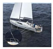
Setting all of the sails and monitoring the sail tension is now almost always fully automated on modern sailing boats. SICK linear encoders integrated in winches and hydraulic cylinders give direct feedback about sail tension and alignment.
