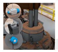
The ladle furnace roof is lifted and lowered, depending on the process step. These mechanical movements are executed by cylinders and drives. Some processes can only be safely executed when the roof is in a defined position. An absolute or wire draw encoder together with a proximity inductive switch care-
