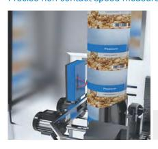
In vertical molding, filling and sealing machines, packaging film is extracted by a roller before being formed and sealed. The SPEETEC 1D non-contact motion sensor reliably detects the speed of the packaging film to ensure the feed has
