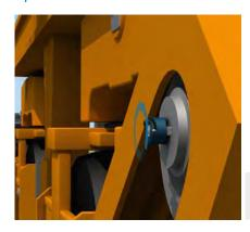
The speed of the drive motor of a crane is measured with the DBS60 incremental encoder. This way, the speed can be con-
