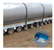
When heavy trucks transport goods, dangerous imbalances can occur, which can lead to the goods slipping or even to the vehicles overturning. To prevent this, sensors are increasingly being used for data acquisition and precise control.
