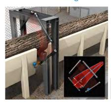
A log measurement system consists of two automation light grids and a DFS60 incremental encoder, and is the ideal solution for determining the log volume – regardless of the surface condition of a tree. The MLG-2 Pro automation light grids also take reliable measurements in extremely harsh conditions, as they are protected by rugged aluminum housing in combination with the IPG2 protective pipe.
