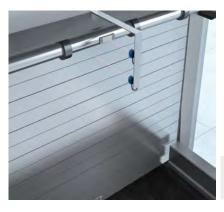
During periods when no luggage is being fed from the collecting belt to the baggage hall, a shutter door secures the baggage hall from unauthorized access. Two G6 miniature photoelectric sensors monitor the opening and closing of the shutter door.
