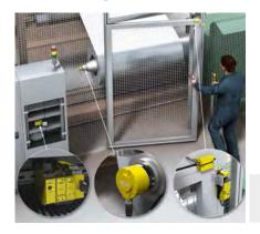
The safe standstill monitoring function only unlocks the locking device when the system has come to a standstill. Thanks to SOS (safe operating stop), the drive does not need to be disconnected from the power supply. Safe Interlocking saves valuable space and ensures maximum productivity: no unnecessary downtimes,
