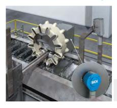
For optimal filling of ingot molds, it is essential to synchronize the speed of the casting wheel with the speed of the ingot casting conveyor. This requires precise measurement of the speed of the casting wheel. The AFS/AFM60
