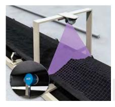
Conveyor belts convey materials throughout all areas of cement plants. They transport raw material and fuels to interim storage facilities and then take steel products and slag to storage areas and to the dispatch points. A conveyor belt malfunction can cause significant delays in production and involve major costs. Therefore it is necessary to monitor the
