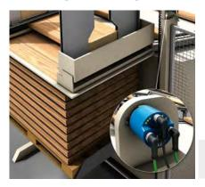
Thanks to its high resolution and IP enclosure rating, the AFM60 PROFINET absolute multiturn encoder determines the position of the stacking unit in the pallet handling machine both reliably and precisely. As a result of its high IP enclosure
