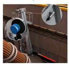
Lances and manipulators for injection, sampling and temperature measurement move in several directions. The entire apparatus moves both up and down, as well as swivels around the vertical axis. The arm carrying the head bearing lance and sampling probe maneuvers up and down, left and right. Such
