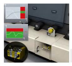
In automated production, plant availability and the safety of operators must be ensured. That is why the Flexi Soft modular safety controller monitors the axis speeds with the FX3-MOC motion
