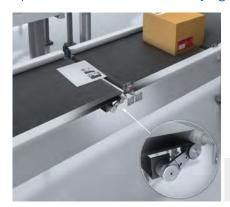
The measured values from programmable encoders can be used to control the conveying speed. They fulfill requirements such as high resolution, maximum repeatability, and support for all mechanical and electrical interfaces.
