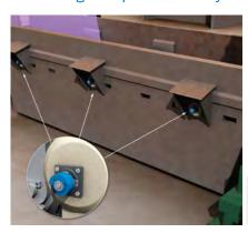
Incremental encoders can control the motor of the hot roller table and therefore also the speed at which steel bars move within the rolling mill train. Controlling the train's speed helps to ensure product quality and to optimize the rolling process. The advantages and
