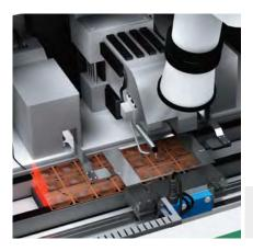
Temperatures are very high in the area around the bonding head, which is why suitably resistant fiber optic systems are advisable in this area. With its mere 16 µs response time, the WLL180T fiber-optic sensor works together with the LL3 fibers to supply the control unit with a precise signal for edge detection. The grippers move the thin lead frames at an extremely high speed, which means Recommended products
