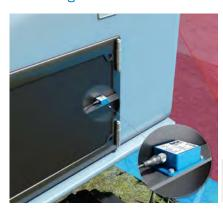
The AHS/AHM36 absolute encoders record the joint position in order to realize automatic swivel movements of the foam monitor, such as the approach into attack position or automatic oscillation
