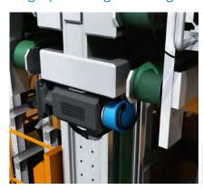
When it comes to the insertion depth, accurate measurements are crucial. A robust absolute encoder on the belt drive with a high resolution and excellent
