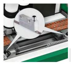
Temperatures are very high in the area around the bonding head, making fiber-optic cable systems the most effective for this application. With its 16 µs response time, the WLL180T works together with the LL3-TH fibers to supply the control unit with a precise signal for edge detection. The grippers of the wire
