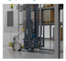
Positioning of the forks of the AGS is handled by constantly-measuring wire
