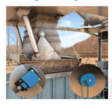
Filling each wagon with coal or metal ore requires precise loading. Too much material results in spillage and waste, while too little is not efficient. The clam shell dispenses the load into the wagon based on its location under the chute. A rugged inductive proximity sensor determines the wagon's exact position while a dura-
