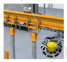
In anode production, the transport carriages of an overhead conveyor system move from one station to another in succession. To avoid banked or empty transport carriages, the conveying speed needs to be monitored. Personnel may also need to carry out work on the
