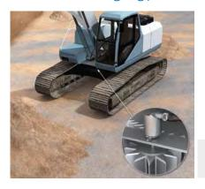
In order to realize semi-automated machine processes it is necessary to measure the position of the upper to the lower carriage with an absolute encoder at the slewing ring. With its very compact size and the rugged design, the AHS/
