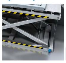
Following machining, residual grids are placed on a scissor lift table. To ensure a smooth transfer, the height of the stack must be aligned with that of the machining table. The analog signal values of the
