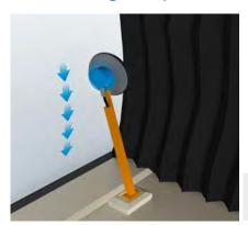
The distance between the aircraft and the ground changes both when boarding and disembarking. The height of the passenger boarding bridge needs readjustment to prevent damage to the aircraft
