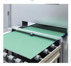
The production of plasterboard requires a very high level of quality. The fast production processes involved demand a reliable speed and length measurement to ensure adherence to the standard dimensions of the plasterboard. SPEE-TEC solves this task reliably without any contact with the product.
