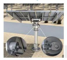
In order to align and adjust the mirrors to best track the sunlight, the heliostat is guided by encoder systems that adjust and identify the exact x and y position of the mirror. SICK manufactures a range of
