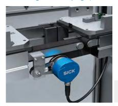
SICK developed an incremental encoder with measuring wheel system specifically to provide slip-free speed measurements on the belt conveyor or dual belt transport system. This makes controlling the assembly line a breeze. Because the
