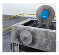
To ensure the empty ingot molds arrive at the casting wheel at the right time and can be filled, it is essential to synchronize the speed of the ingot casting conveyor with the speed of the casting wheel. This requires precise measurement of the speed of the ingot casting conveyor. The DBS36 Core incremental encoder performs this task reliably in the harsh environment of aluminum casting.
