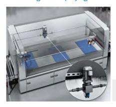
The product travel path of the spraying unit is adapted to the dimensions of the corresponding furniture board using the AFM60 EtherCAT® absolute encoder. This
