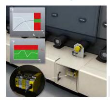
The modular Flexi Soft safety controller is responsible for monitoring all safety functions in the production system. When combined with the Flexi Soft Drive Monitor and the DFS60S Pro safety
