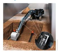
When space is limited, precise control of the excavator arm is important to prevent damage to the surrounding infrastructure and pipelines in the ground. With the MAX® linear encoders - integrated in the four hydraulic cylinders of the excavator - indirect measurement of the position of
