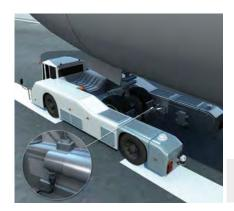
It is important to check the exact position of the nose wheel receptacle flap in the nose wheel receptacle. The singleturn type of the AHS/AHM36 absolute encoder is used for this purpose. It can also be used in harsh ambient conditions thanks to its rugged and reliable fully magnetic
