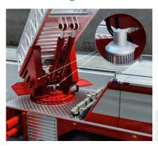
The angle and the position of the aerial ladder relative to the lower carriage must be known in order to realize repeating motion sequences. The AHS/AHM36
