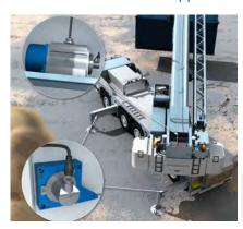
A sub-function for the load torque restriction on the mobile crane is the position detection of the extendable support feet and the recording of the boom and crane arm position. The wire draw encoders from the EcoLine product family are per-
