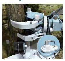
The rugged and highly compact AHS/ AHM36 absolute encoders determine the gripper position to measure the tree-trunk diameter. A further encoder detects the feed rate, thereby measuring the length of the trunk.
