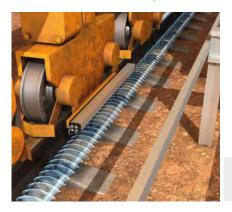
The non-contact KH53 linear encoder for measuring length makes it possible to detect the position of the crane portal precisely over a distance of up to 1,700 m. Thanks to the absolute position de-
