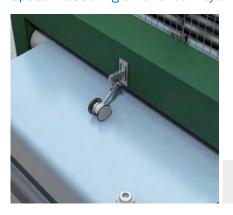
The DFV60 incremental measuring wheel encoder uses a friction wheel to measure the exact feed speed of the
