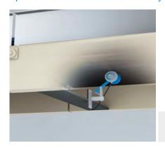
A DFV60 high-resolution, incremental measuring wheel-encoder installed under the conveyor belt provides information about the transport speed of a piece
