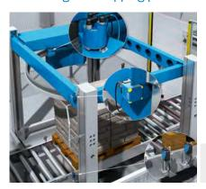
After the pallet has reached its position, the stretch film is secured to the pallet and wrapped using upward and downward movements of the film. SICK's measurement technology products handle both the measurement of pallet dimensions and detection tasks for controlling
