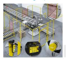
A casting system for aluminum ingots has various dangerous parts, such as the rotating casting wheel, conveyor belts, as well as automated grippers or robots. The molten metal and hot surfaces also pose a hazard. A combination of several safety sensors and MOC Motion Safety Drive Monitor ensure safe machine
