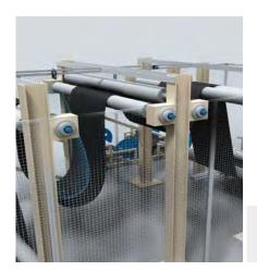
Loop control enables the uncoupling of processes such as calendering and material in-feed and out-feed. The distance sensors installed above the loop are used either for continuous measurement with analog output or with two previously taught-in digital switching points. The loop measurement is per-formed with only one sensor per loop, which reduces the installation work required. Depending on the properties of the material and
