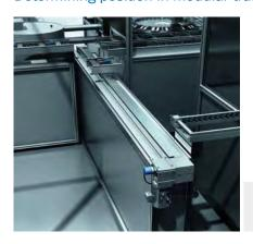
For the flexible adaptation of modular transfer systems to different assembly systems, these transfer systems incorporate the use of what are known as right angle transfers, cross transfer belts or shuttle units. These elements make it possible to rotate the workpiece carriers 90 or 180 degrees. This repositioning of the carriers is typically carried out
