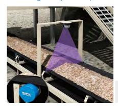
Conveyor belts transport raw material deliveries to interim storage facilities and then take steel products and slag to storage areas and to the dispatch points. A conveyor belt malfunction can cause significant delays in production and involve major costs. It is therefore necessary to monitor the operation of
