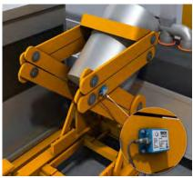
When connecting the anode block and support, liquid cast iron is used as an "adhesive." The cast iron is poured from a pot into the space between the support and the anode block using a tilting device. In order to properly pour the liquid iron, it is necessary to know the precise position of the tilting device. The TMS/TMM88 inclination sensor
