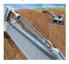
Positioning the individual hydraulic cylinders of the excavator arm enables partial automation of work processes. This makes it possible to strip a slope, for example. Rugged MAX® linear encoders
