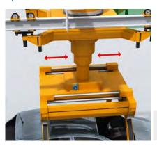
The electrical overhead conveyor brings the car bodies to designated workplaces. The speed is specified by the higher-level control; an incremental encoder determines the speed. In case of requirements for secure speed, the DFS60S Pro assists with the realization of collision protection in combination with a safety laser scanner.
