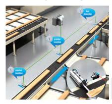
In conjunction with a DFS60 incremental encoder, the PowerProx Speed MultiTask photoelectric sensor identifies the position and length of the wooden boards when they pass through. Each
