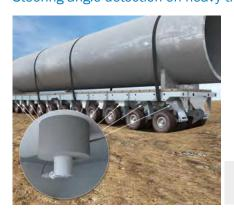
For simpler and more reliable maneuvering of heavy trucks carrying large payloads, many of these vehicles have sensors for controlling the steering angles of each individual drive axle. The AHS/AHM36 absolute encoder is ideally suited for this task. With its IP 66/IP 67
