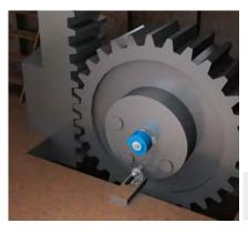
The vessel or shell of a basic oxygen furnace is mounted in a way that allows tilting movements. Depending on the process step during heating (e.g. tapping, de-slagging, charging), the shell must be tilted in different positions by means of hydraulic cylinders. To control the tilting process, measurement equipment pre-
