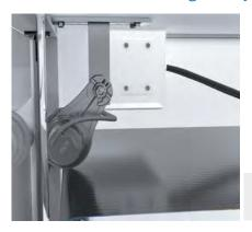
The actual speed is a significant parameter for the precise control of a system such as a code printer. The DBV50 Core measuring wheel encoder measures the exact speed of the packaging film. With its high resolution of up to 2,500 pulses per rotation, it supplies the system with precise speed signals.
