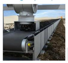
When the actual speed of a conveyor belt differs from the required speed, production yield changes and production steps can be misaligned. Maintaining the proper speed and taking periodic measurements to prevent interruptions or failures are therefore essential for maintaining production throughput. A safety encoder continuously monitors conveyor belt operations to maximize performance, while an encoder for functional safety furthermore supports safety functions.
