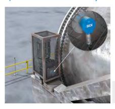
The aluminum recovered from recycling of aluminum waste is first placed in a furnace, usually a rotary drum furnace. The rotation of the furnace chamber ensures a perfect mixing of the input materials and accelerates the smelting process.
