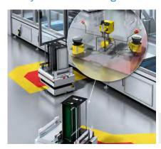
Automated guided carts (AGC) manage high speeds even when going around curves thanks to the switching of protective fields. Reliable detection of speed and direction of travel with safety solutions from SICK also reduces the number of components and thereby the required installation space in AGCs.
