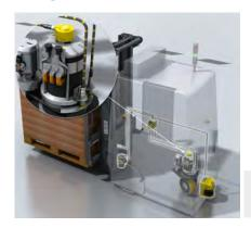
AGVs for automated goods transport are equipped with a wide range of sensors depending on the requirement. A safety system consisting of safety laser scanners, safety controllers and safe encoders enables non-contact monitoring of the travel path and adjusts the speed and direction of movement. Inductive proximity sensors or wire draw encoders detect the end positions of lifting forks.
