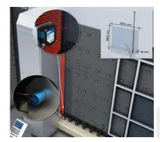
A system composed of the MLG-2 Pro automation light grid, the DBS36 Core incremental encoder and the OD5000 displacement measurement sensor measures the glass plates as they are moving. The outer contour is calculated using the height information recorded by the MLG-2 Pro and the speed signal from the DBS36 Core. The thickness of the glass is detected without making contact and with maximum precision with the OD5000.
