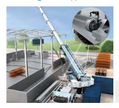
Space is often tight in construction sites in cities in particular. MAX® linear encoders are integrated into the hydraulic cylinders of the four crane supports and help to position them precisely. This makes it possible to extend all four supports,
