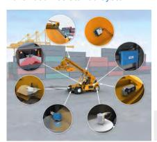
Intelligent assistant systems prevent hazardous states arising from the load level of a vehicle or the driving behavior of the driver. These modular systems can be used to provide either active or passive assistance. Whereas active assistance systems directly intervene in the motion
