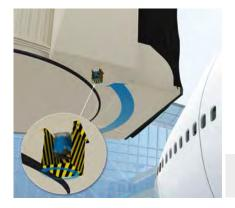
The AFS/AFM60 PROFINET absolute encoder determines the rotation of the passenger boarding bridge"s bridgehead rotation system. The encoder"s data
