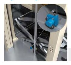
Following machining, residual grids are placed on a scissor lift table. To ensure a smooth transfer, the height of the stack must be aligned with that of the machining table. The analog signal values of the
