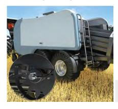
The compact AHS/AHM36 absolute encoder can determine bale length on square balers. By detecting the absolute position of the measuring wheel, the encoder determines the feed rate, and,
