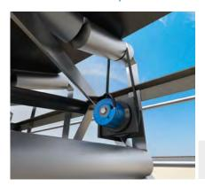
The belt speed at which excavation materials are conveyed to stockpiles, ship loaders, and railroad loading facilities is of paramount importance. The DFS60 incremental encoder calculates the speed and running direction of the belt. The
