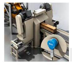
The AFM60 SSI absolute multiturn encoder reliably signals the precise position of the machine to the system control. With magnetic scanning, rugged housing,
