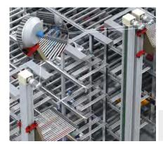
The AHM36 absolute encoder provides the data to position the lift with high accuracy and high repeatability. The encoder is available with CANopen, IO-Link or SSI interface - depending on the used control architecture of the early baggage accumulator. Intelligent diagnostic functions enable evaluations
