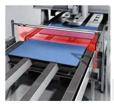
In combination with the DFS60 incremental encoder, the MLG-2 Pro measuring automation light grid measures the width, length, and position of the moving
