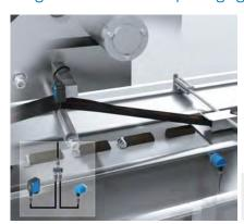
The AHS/AHM36 IO-Link Advanced absolute encoder, in combination with a print mark sensor, measures the exact length of packaging film. With the help of the integrated A30 Smart Task, after a set length value passes through, a trig-
