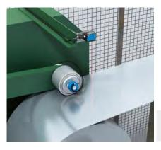
To ensure a constant feed of material, the uncoiling speed of the sheet coil must be regulated. The distance sensor continuously measures the radius of the sheet coil throughout the entire unwinding process. The DBS60 Core incremental encoder uses a friction roller
