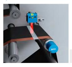
When changing the roll, the beginning and end of two consecutive rolls are joined together using splicing tape. Color, contrast, luminescence, and glare sensors from SICK detect the tape. As a
