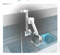
The position of the wafer carrier can be determined reliably with absolute encoders: with the AFS60 Singleturn on the vertical and the AFM60 Multiturn on the horizontal axis. Thanks to the fieldbus and Industrial Ethernet interface.
