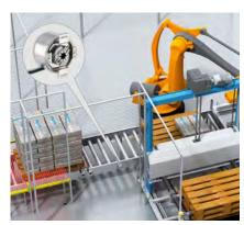
Automatic palletizers stack the filled cement bags onto pallets. The DFS60 incremental encoder monitors the trans-
