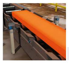
Positioning the cutting torch during the continuous casting process is an important step in guaranteeing that each object is precisely cut to length. An encoder and presence detection sensor enable accurate positioning of the cutter as the hot steel is being extruded. While the photoelectric switch detects
