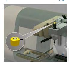
For stand-alone machines such as a drilling machine, the user is protected from the hazardous point by a safety door or hood. For set-up operation, the speed of the drilling arm and of the tool table
