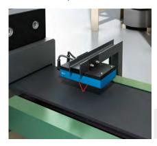
When extruding tire rubber, the belt thickness of the tire material must be adhered to exactly in order to ensure product quality of a consistently high standard. This requires precisely synchronizing the release speed of the tire material on the belt to the continuous
