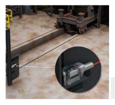
Ladle cars transport ladles to different locations within the steel plant. The plant's central control room must know where individual ladle cars are and if they are correctly positioned at each location. Missing or improperly positioned ladle cars can lead to inefficiency and even catastrophic consequences. Track-
