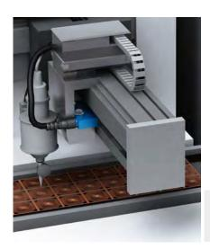
In chip bond machines, defined chips and small rectangular plates from the wafer are bonded to lead frames. If the adhesive is not positioned exactly on the lead frames, the semiconductor chips will be unusable. Incorrectly positioned adhesive points need to be detected before the chip is put in place. The 2D vision sensor Inspector increases the availability of the bond machine. The Inspector can define up to 32 different reference images with up to 16 switch-
