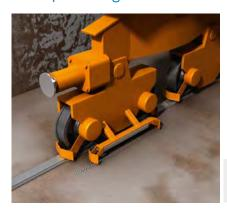
A non-contact KH53 linear encoder with a resolution of 0.1 mm and optionally for measurement lengths up to 38, 107, 354, and 1700 m is used for detecting the position of the crane portal. The KH53 is wear-free and is also ideal for harsh ambient conditions.
