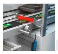
The DBS60 incremental encoder transfers the position of the belt for synchronization of both sensor signals. Alternative-
