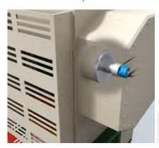
An AFS60 absolute encoder is mounted to the eccentric shaft on mechanical presses for the purpose of determining the position of the press stroke. It reli-
