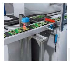
The WLL180T fiber-optic sensor in combination with the LL3-TS fibers is ideal for detecting the front edges of printed circuit boards on conveyor belts. This system supplies the position data
