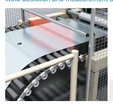
The MLG-2 Prime automation light grid detects a hole less than 15 mm in size that marks the weld of the coil. The DFS60 incremental encoder determines
