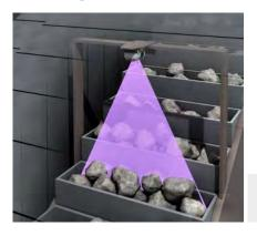
After the burning process, a bucket conveyor transports the hot clinker to the interim storage area. Belt malfunctions can cause significant delays in production and involve major costs. It is therefore necessary to monitor the operation of all conveyor belts, as well as the proper loading, unloading, and position-
