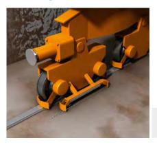
Precise crane positioning can be achieved by using the rugged KH53 linear encoder. To properly determine the crane's x-axis, this non-contact, virtually maintenance-free linear measuring system mounted on the crane's column. This encoder determines the crane's absolute position by sensing the integrat-
