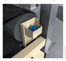
The conveyor belt speed at which the biomass is transported to the shredder and then to the storage location is very important when it comes to controlling the material flow. The DFS60 incremental encoder calculates the speed and
