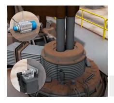
A ladle furnace's electrodes are hoisted and lowered by electrode arms. In some cases, the electrodes' position determines other movements or timing of subsequent steps, such as moving the ladle. Therefore, knowledge of the electrodes' exact position is imperative for safe and
