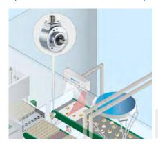
The DBS60 Core incremental encoder measures the speed of the belt. Pralines of different types are transported on the belt and sorted into the trays with a Pick
