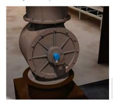
Rotary valves control the carbon and sinter supply for the subsequent processing steps. Encoders control the rotary valve motor and therefore the amount and speed at which carbon and sinter material is supplied to the subsequent processes. The fact that the encoders
