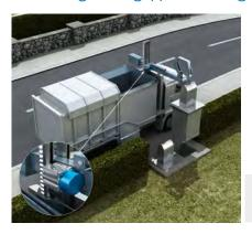
The exact position of the gripper arm must be recorded to enable automatic emptying of waste containers. Therefore the compact AHS/AHM36 absolute encoder determines the rotational movement on the gripper arm. Thanks to the
