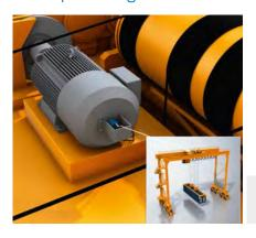
Several combined encoders enable the correct positioning of the crane harness. Linear encoders are used for precise control of the horizontal axis movements, a rugged multiturn absolute encoder is employed to position the lifting axis: Any
