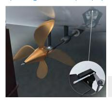
Controllable pitch propellers are used when good maneuverability, generator operation and/or varying continuous speeds are required. The propeller blades are fixed to the hub and can rotate. Linear encoders are placed in hydraulic cylinders that act on the shaft for
