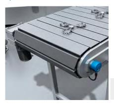
In order to synchronize the product transport with subsequent processing steps, an encoder mounted directly on the drive shaft must measure the conveyor speed. The rugged DBS60 Core incremental
