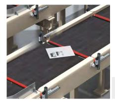
The leading edge detection serves to convey objects at a specified distance from the belts to the main sorter. The combination of high-resolution light grids and high-resolution encoders allows leading edge detection and the detection of additional object profile information such as the length. The duration of the
