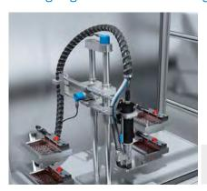
To guide screw guns at precise angles, the carrying arms for the horizontal projection and the rotation axis are each equipped with an AHM36 absolute encoder. This ensures that components are screwed together in the accurate position.
