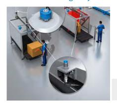
Two 2D LiDAR sensors on a positioning unit are evenly maneuvered over the cargo to provide space-saving static measurement of individual freight objects that are not positioned on a load carrier. Two LMS4000 scanners record two-dimensional scan data of the cargo. A DFS60 incremental encoder provides
