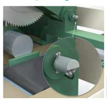
The height of the saw blade is automatically positioned for optimum control of the sawing process. The DBS36 incremental encoder supplies precise measurement values for this purpose. It
