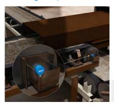
The conveyor belt used to supply and transport carbon and sinter must be monitored and maintained in order to avoid spillage, down time and material waste. An inductive sensor's robustness in very harsh environments and its high
