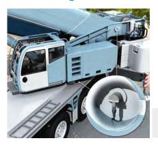
The angle and the position of the boom relative to the lower carriage must be known for a stable load torque restriction. The absolute encoder
