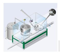
The precise position and speed monitoring is handled by an A3M60 absolute encoder. The encoder is connected directly to the carousel wheel via gear stages. The resolution per rotation depends on the number of filling stations. The number of encoder rotations
