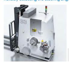
In order to adapt the automated guided vehicle's protective fields to its exact driving scenario, the steering angle must also be captured by the drive and steering drives. When the MOC1 Flexi
