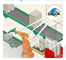
AFM60 Multiturn absolute encoders transmit the absolute positions of the
