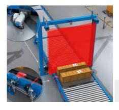
Two LMS5xx 2D LiDAR sensors installed above the conveyor belt scan the freight during transit through the measuring system. A three-dimensional image is produced using the two-dimensional scan data from the LMS5xx scanners and the precise speed data of the DFS60
