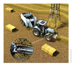
Precise positioning of the control for steering is a basic prerequisite for autonomous driving of mobile machines. The MAX® linear encoder - integrated in the steering cylinder of the tractor - detects
