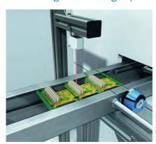
Minimizing soldering faults is a constant aim in PCB production. Selectively checking the height of critical components before and after the soldering process minimizes many faults. With the OD Mini displacement measurement sensor and DBS60 Core encoder, this can be achieved in a quick, flexible, and above all cost-effective manner.
