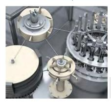
The carousel angle of rotation serves to control the transport of bottles through the blow stretching machine. A high-precision AFM60 EtherCAT® absolute encoder, which precisely synchronizes the rotations electronically, supplies the
