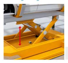
The scissor lift table brings the powertrain with the drive unit to the correct height position for installation on the car body. The compact BKS wire draw encoder measures the height precisely and passes this on to the scissor lift table controller via the SSI interface.
