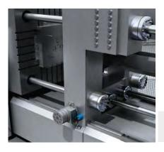
In order to produce the locking force necessary for a closed mold, the closing stroke of the machine must be matched to the current mold height, which can differ for each individual mold. To achieve this, it must be possible to move the entire mold-closing unit lengthwise. This typically occurs by means of a mold height adjuster that is powered by a
