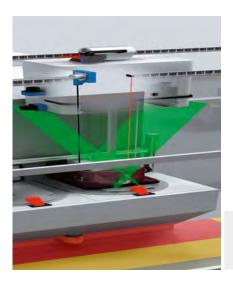
The risk of material breaks in expensive semiconductor wafers must be kept as small as possible. To ensure this is the case, sensors are used, monitoring, for example, whether a FOUP (Front Opening Unified Pod) is jittering too much when being lowered. The miniature photoelectric sensor WL100L detects these kinds of unwanted movements. As a Class 1 laser sensor, it poses no risk to the operator. The EcoLine wire draw encoder, lightweight at just 180 grams and also
