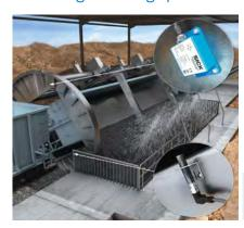
Efficient, fast unloading of filled wagons via a tippler mechanism is required for maximum productivity. Determining the wagon's precise position for the tippler mechanism to properly function is essential. An interlinking system of rugged
