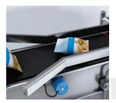
The conveyor belt speed needs to be determined for accurate control of the transport distance between packages. This is necessary in a variety of machines. Potato chips are fed into the machine from above. The packing film is removed from a roll, shaped, and sealed. A conveyor belt then transports the packaged product to the following process step. The
