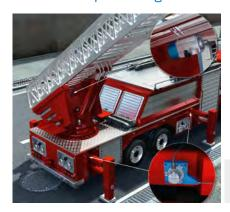
Sensor solutions for position recording are used to realize reproducible motion sequences of the aerial ladder. Wire draw encoders from the HighLine product family detect the length of the extended ladder. Thanks to robust mechan-
