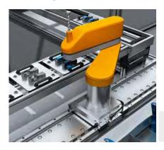
The SCARA robot must move in sync with the conveyor speed so that it can remove the workpieces from the belt. The TTK70 linear encoder determines the absolute position of the SCARA robot. This encoder consists of a compact read head and a piece of magnetic tape that serves as a reference scale. The non-contact principle of operation means that the position is determined without causing
