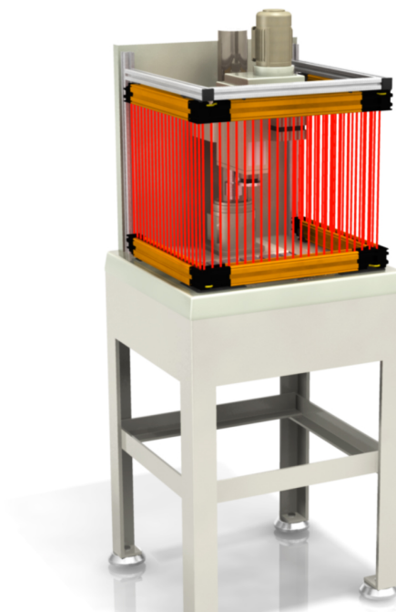
Figure 38. Cascaded light screens guarding a u-shaped cell
