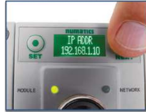
Graphic Display for Configuration & Diagnostics
