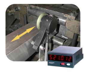
If you're looking for a quick and simple position monitoring system... Look no further! The 520 display along with the Tru-Trac with quadrature output provide a simple solution. The compact size of both units make for easy mounting and setup!
