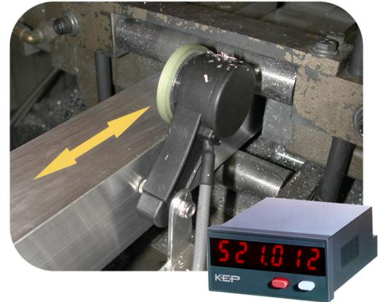
If you're looking for a quick and simple position monitoring system... Look no further! The 520 display along with the Tru-Trac with quadrature output provide a simple solution. The compact size of both units make for easy mounting and setup!
