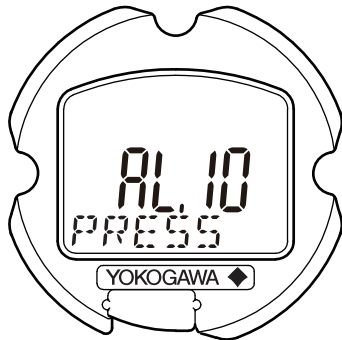
Self-diagnostic error on the integral indicator (Faulty transmitter) F0702.ai
