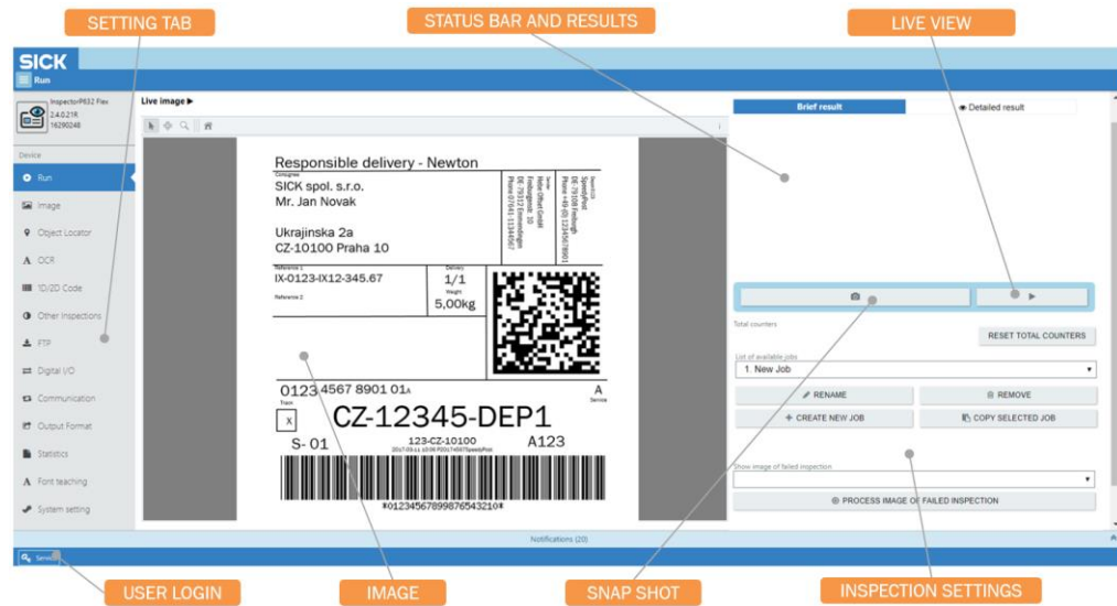
Figure 7 Label Checker GUI
