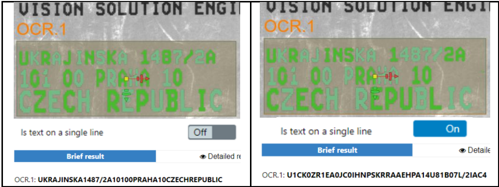
Figure 65 Is text on a single line - enable/disable
