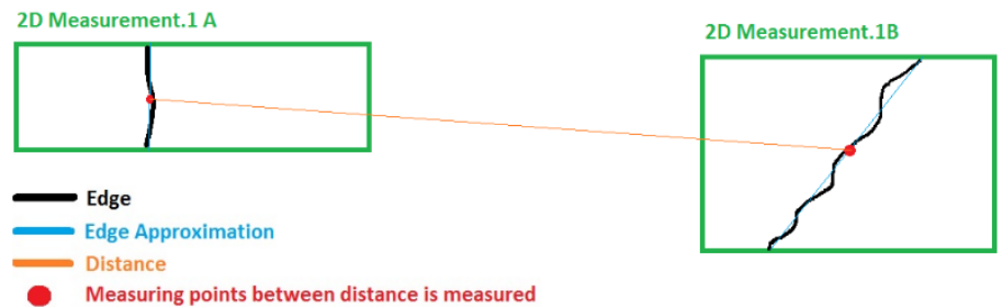
Figure 81 Euclidean distance - 2D Measurement
