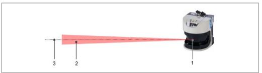
Fig. 10: LMS5xx beam expansion
