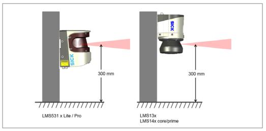
Fig. 93: Installation situation (open space protection)\*
