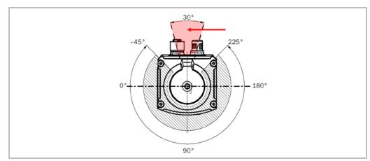
Fig. 23: Area behind the reference target in which no reflective surfaces are allowed
