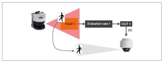
Fig. 67: Field-based switching of cameras (overview)
