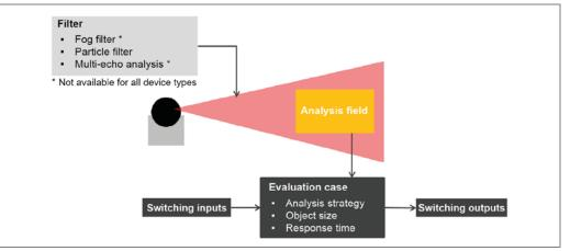
Fig. 32: Filter - analysis fields - analysis cases - switching inputs
