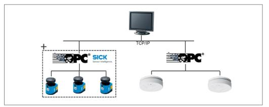
Fig. 79: Integration of laser scanners using SICK OPC server
