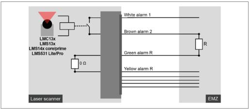
Fig. 64: Circuitry with resistance monitoring (LMC13x/LMS13x/LMS141 core/LMS14x prime/LMS531 Lite/LMS531 PRO)
