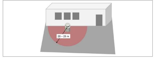
*Fig.* 91: LMS1341x core/prime monitored area (open space protection)
