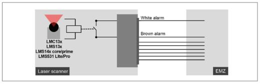
Fig. 62: Circuitry without resistance monitoring (LMC13x/LMS13x/LMS141 core/LMS14x prime/LMS531 Lite/LMS531 PRO)
