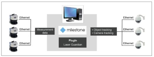
Fig. 71: How to integrate a laser scanner into Milestone XProtect
