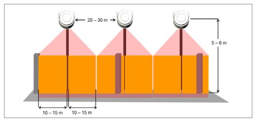
Fig. 83: LMS13x monitored area (fence protection)
