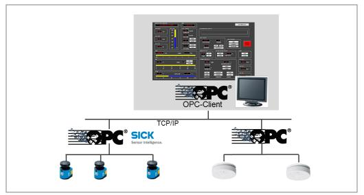
Fig. 80: Viewing information based on OPC
