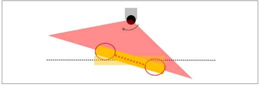
Fig. 43: Protection against tampering thanks to contour as reference
