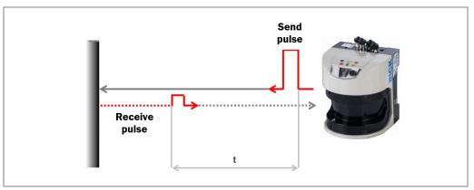
Fig. 2: Pulse time-of-flight measurement principle of operation
