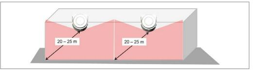
Fig. 86: LMS14x core/prime monitored area (facade protection)
