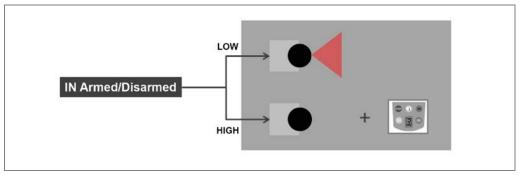
Fig. 59 Switching the laser scanner to sharp/not sharp (switching input Armed/Disarmed)
