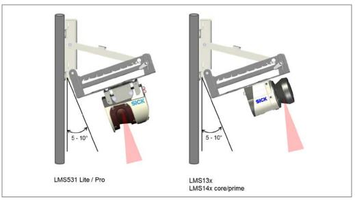
Fig. 84: Installation situation (fence protection)\*
