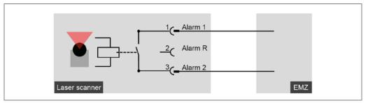
Fig. 61: Circuitry without resistance monitoring (LMC12x/LMS12x)
