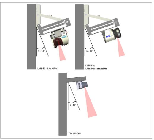
Fig. 89: Installation situation (facade protection)\*
