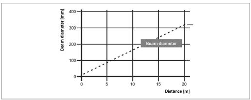
Fig. 9: LMS1xx beam diameter
