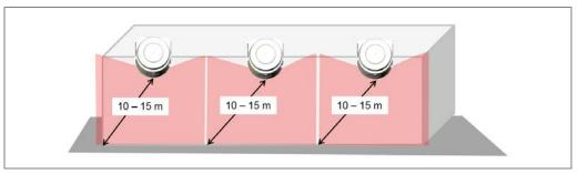
Fig. 87: LMS13x monitored area (facade protection)
