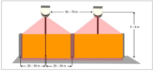
Fig. 81: LMS531 Lite/PRO monitored area (fence protection)
