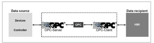
Fig. 78: OPC client/server architecture
