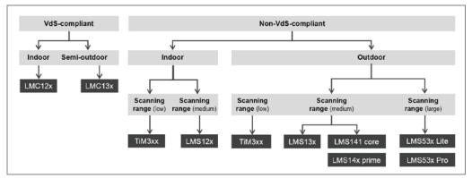
Fig. 20: Flowchart for device selection
