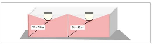
Fig. 85: LMS531 Lite/PRO monitored area (facade protection)
