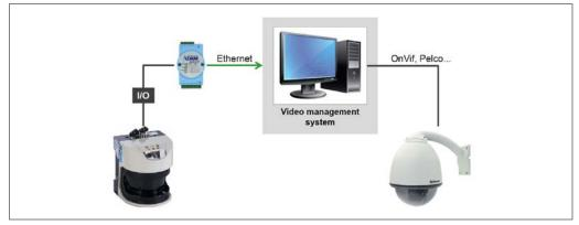
Fig. 69: Field-based camera control (via video management system)
