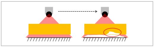
Fig. 46: Field breaches caused by changing ambient conditions
