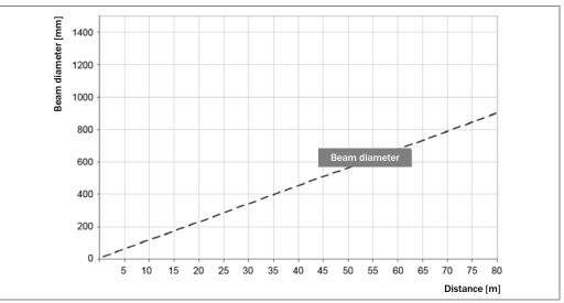
Fig. 11: LMS5xx beam diameter
