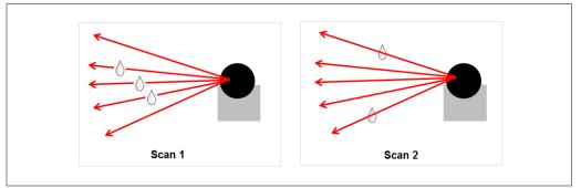
Fig. 33: Particle filter principle of operation
