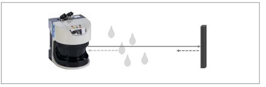
Through the reception of several echoes for each emitted laser pulse, object detection can be optimized and refined significantly.
