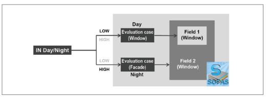
Fig. 58: Activating analysis cases (switching input Day/Night)
