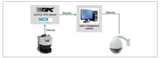
Fig. 70: Field-based camera control (via OPC)
