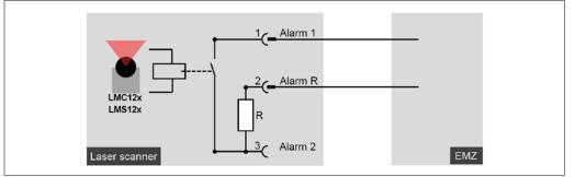
Fig. 63: Circuitry with resistance monitoring (LMC12x/LMS12x)
