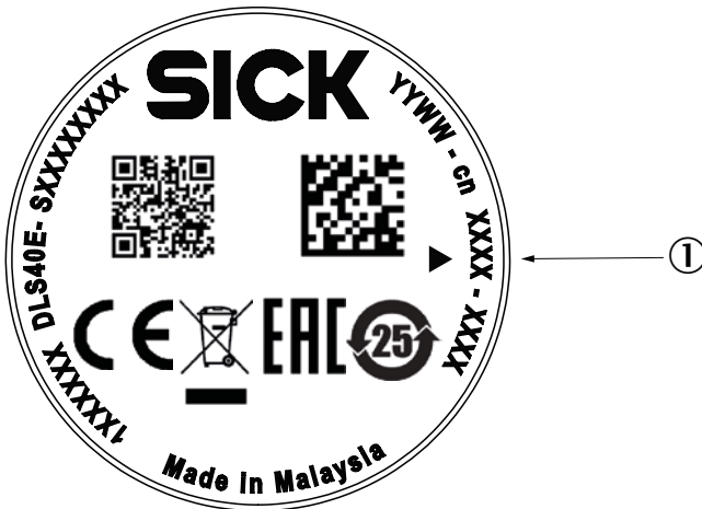
① Zero pulse mark on housing
