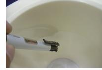
Surface of ceramic liner tube (mirror finished)
